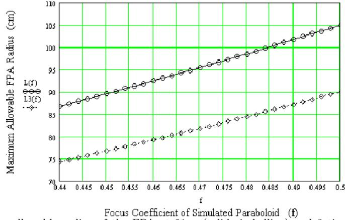
Fig. 5 The allowable radius of the FPA at 21cm(solid circledline) and 3 times allowable radius at 6 cm (dashed diamond line) vs. the focus coefficient of the FAST
