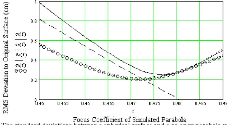
Fig. 1 The standard deviations between a spherical surface and a co-apex parabola within an aperture of 300m calculated with both cosine approximation and exact formula respectively
