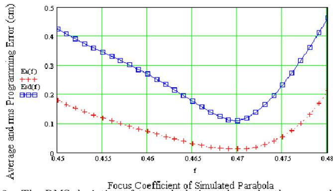
Fig. 3 The RMS deviation of two calculations shown by the squared-solid curve and the average square discrepancy indicated by the crossed-dashed curve
