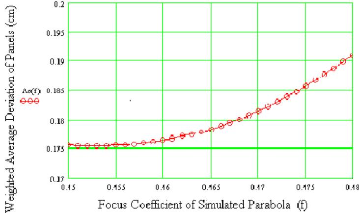
Fig. 2 The weighted average of the standard deviation of spherical panels to parabola vs. focus coefficient between 0.45 and 0.48
