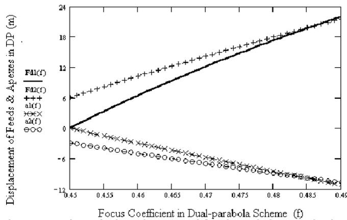
Fig. 4 Displacements of two feeds and apexes of fitted parabolas vs. the focus coefficient between 0.45 and 0.49 in the dual-parabola fitting scheme
